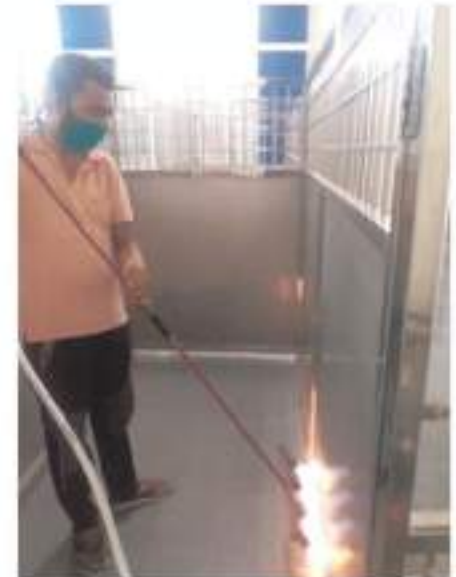
Picture 10: Flaming of SS Steel Kennels (2)
